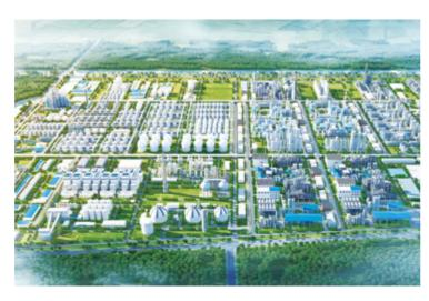
SUEZ provides process design, equipment and material supply as well as technical services for the wastewater treatment plant of Shenghong Petro in Xuwei Petrochemical Industrial Park in Lianyun Port. The plant's treatment capacity is 79,200m<sup>3</sup>/day.
